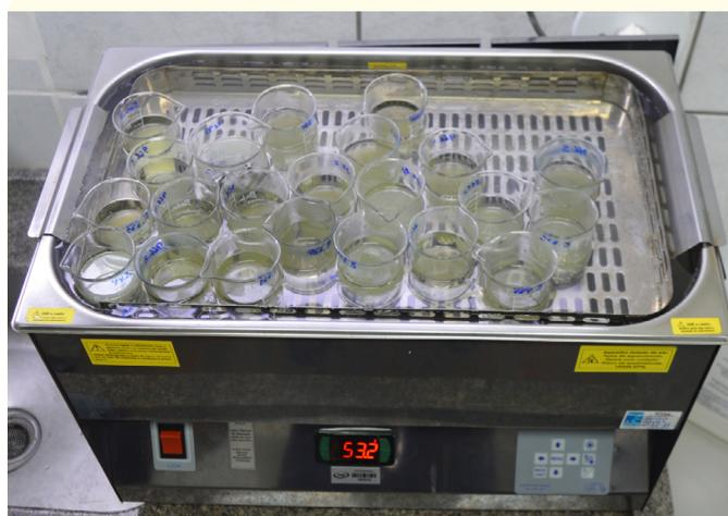
**Figure 5:** Implants under the first asepsis (ultrasonic tank).
